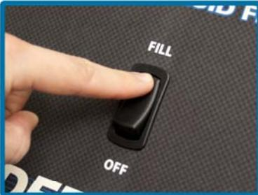
Move switch on the front panel of the machine in the "FILL" position. The pump will begin to run in bypass when the switch is actuated.
