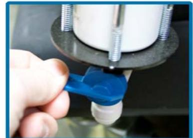
The water bath can be easily drained and refilled using the ball valve at the bottom of the tube. Simply fill the tube with water and open the ball valve to drain it and periodically change the water in the bath.
