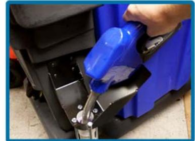
When DEF fill is complete, place the nozzle back into the water bath on the side of the machine to ensure proper function of the vacuum shutoff.
