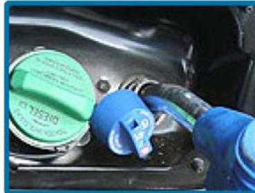
Using the nozzle, fill the vehicle's DEF reservoir with new DEF fluid. The nozzle has a built in vacuum shut off feature that will shut off the flow of DEF when the vehicle's reservoir is full.
