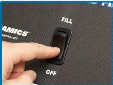
Return switch on the front panel of the machine to the "OFF" position.
