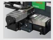
Built to last — Machine shop quality dovetail way and adjustable gibb design
