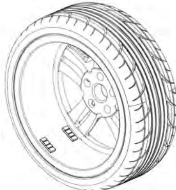
The two adhesive weights must be securely applied in order to execute two measurements using the automatic distance and diameter gauge and two laser spotter positions using the on-screen buttons.
