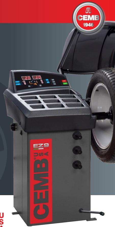
MULTIFUNCTIONAL DIGITAL PANEL with Direct Weight Placement program and Behind Spoke (Split) mode
