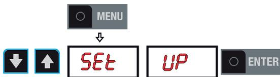
1. Press to view the diameter gauge CALIBRATION function.
