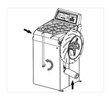
10. At this stage, return the start lever to the start posi tion and release the start button. When unbalance values are displayed, tyre rotation can be halted using the start roller
