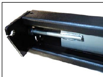
14. Stand-up and arrange the two end structures (Columns & Crossbeams) so that the outside of the cross rail to the outside of the cross rail measurements are close. Compare the measurements from the left and the right until they are diagonally within 1/2". The 1/2" variance will help in mounting the runways.
