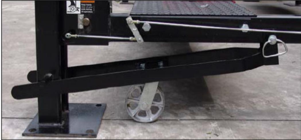
4. Lower lift and the columns will automatically raise off the floor.
