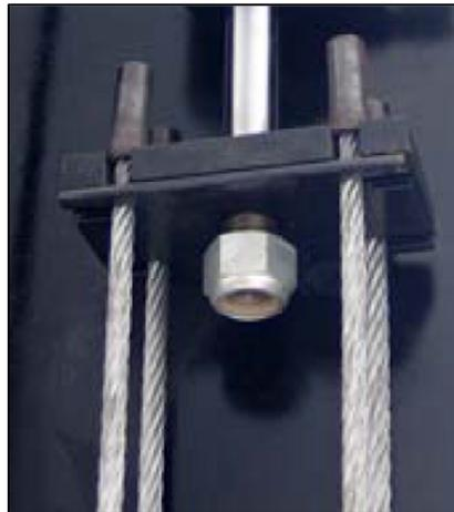
6. Locate the four cable ends and route the appropriate Cable through each hole in corners of the Mainside Runway, shown in Figure # 4. Take up as much cable slack as possible and lay each cable back into the runway. **Note:** Make sure that cables are properly routed around pulleys and are not in a bind. Refer to Figure 4 for Cable routing detail.
