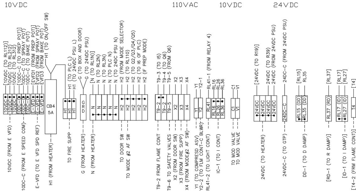
IF ANY OF THE ORIGINAL WIRE AS SUPPLIED WITH THE HEATER MUST BE REPLACED, IT MUST BE REPLACED WITH TYPE THHN [194F (90C)] WIRE OR ITS EQUIVALENT.
