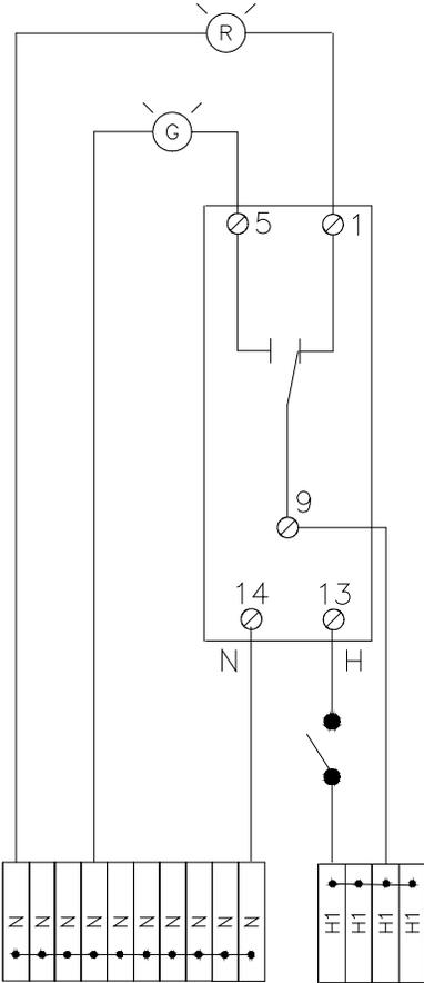
Relay terminals follow a numbering system. Please take a look at the Relay Terminals drawing. Make sure you always check the relay terminal layout specs if you are not sure what a terminal does. There are differences in terminal numbers based on different brands and based on number of poles. For example 13 and 14 are not always the coil terminals.
