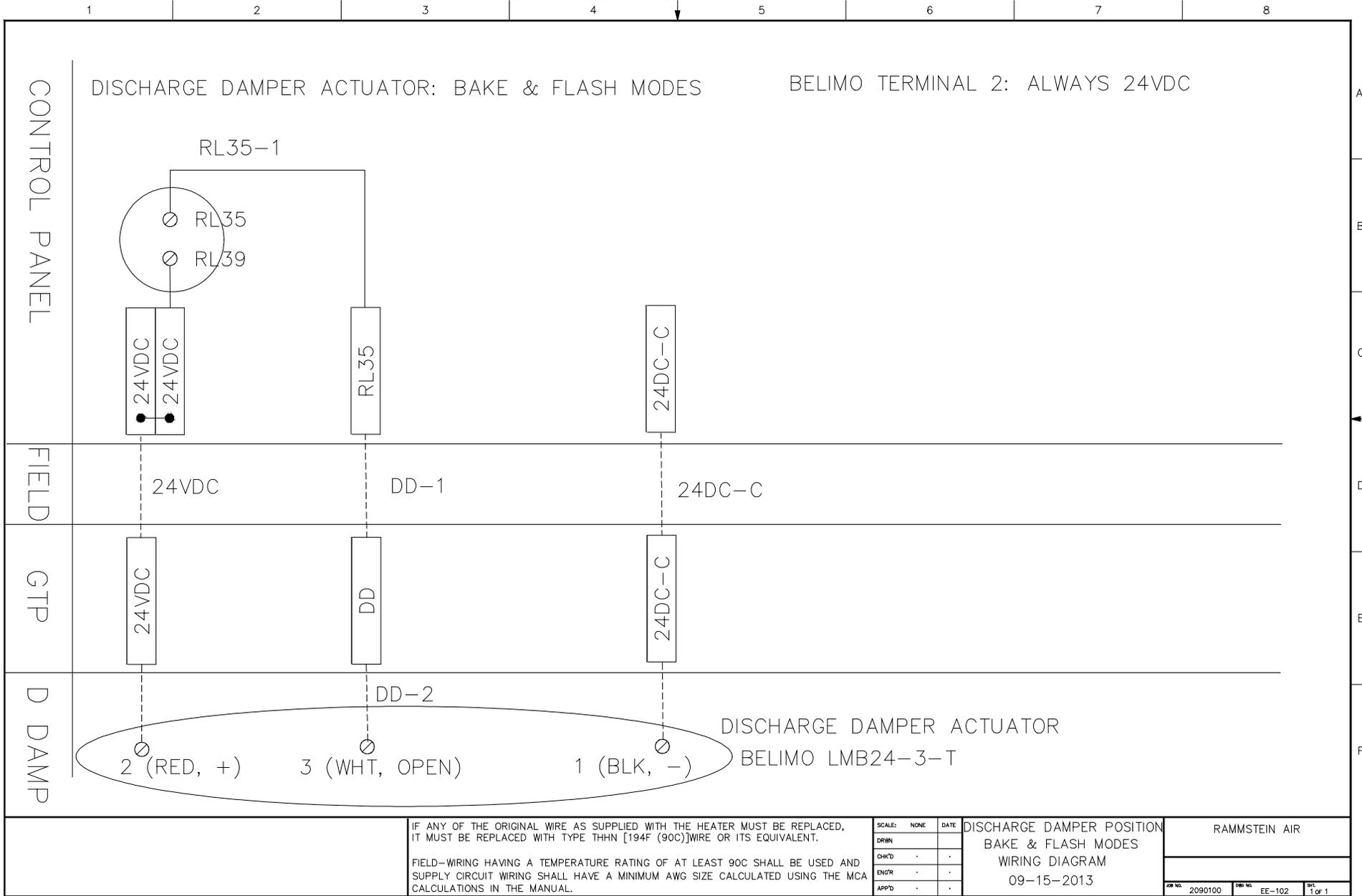
IF ANY OF THE ORIGINAL WIRE AS SUPPLIED WITH THE HEATER MUST BE REPLACED, IT MUST BE REPLACED WITH TYPE THHN [194F (90C)] WIRE OR ITS EQUIVALENT.
