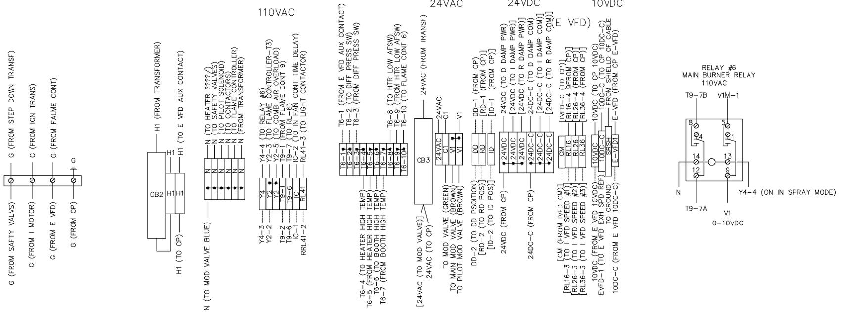
IF ANY OF THE ORIGINAL WIRE AS SUPPLIED WITH THE HEATER MUST BE REPLACED, IT MUST BE REPLACED WITH TYPE THHN [194F (90C)] WIRE OR ITS EQUIVALENT.
