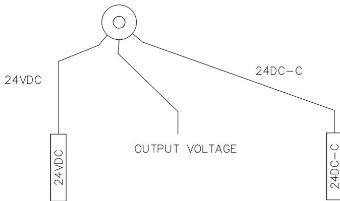
Measure DC on the center terminal while turning the potentiometer L to R.
