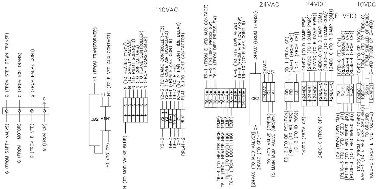
IF ANY OF THE ORIGINAL WIRE AS SUPPLIED WITH THE HEATER MUST BE REPLACED, IT MUST BE REPLACED WITH TYPE THHN [194F (90C)] WIRE OR ITS EQUIVALENT.
