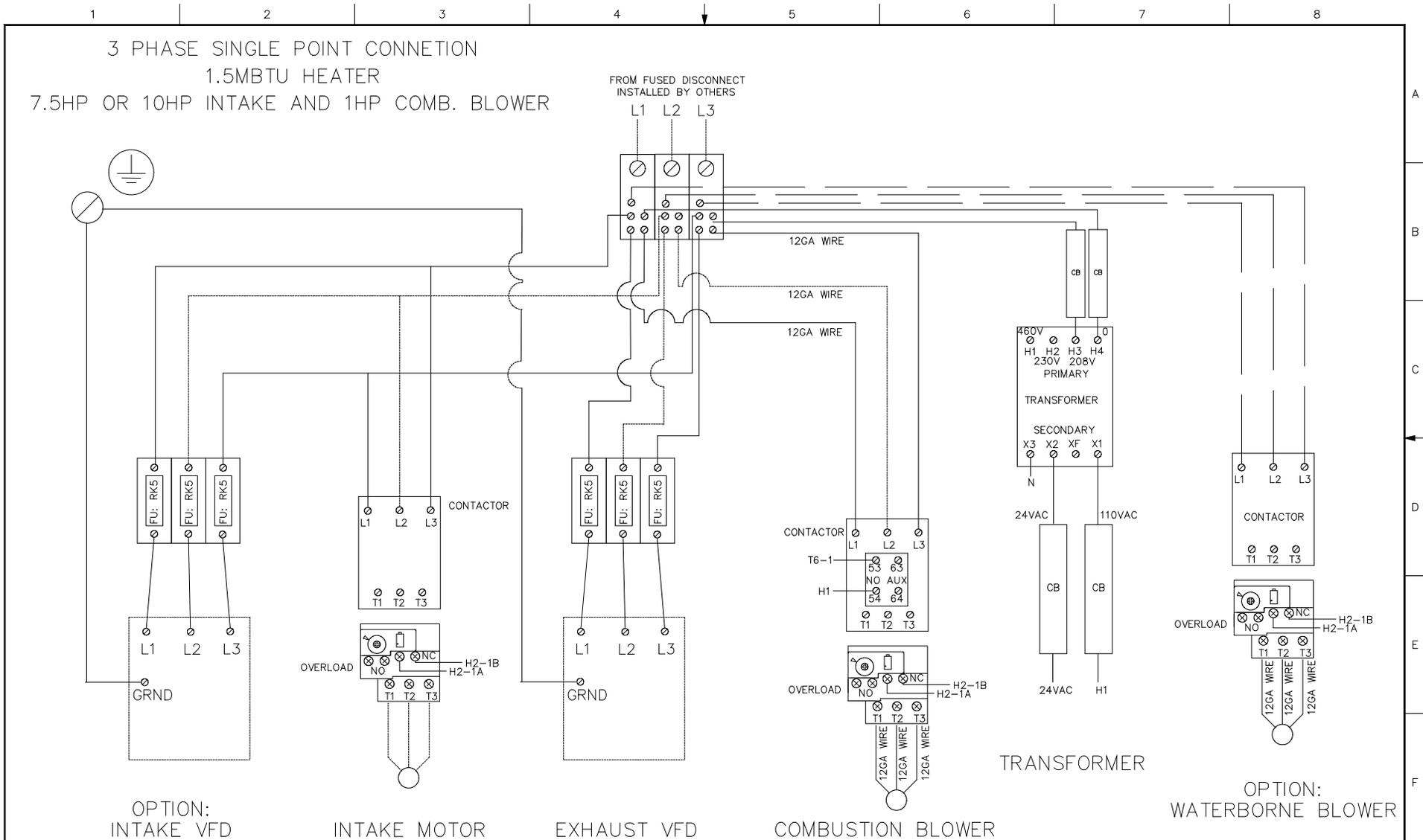
IF ANY OF THE ORIGINAL WIRE AS SUPPLIED WITH THE HEATER MUST BE REPLACED, IT MUST BE REPLACED WITH TYPE THHN [194F (90C)] WIRE OR ITS EQUIVALENT.
