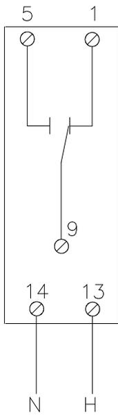
2. Wire a switch to activate the relay
