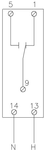
Relays have coil terminals. When the coil is energized the relay contacts change positions. Relays are voltage specific. For example, some relays are turned on by 110V, some by 12VDC, some by 24VAC, etc.
