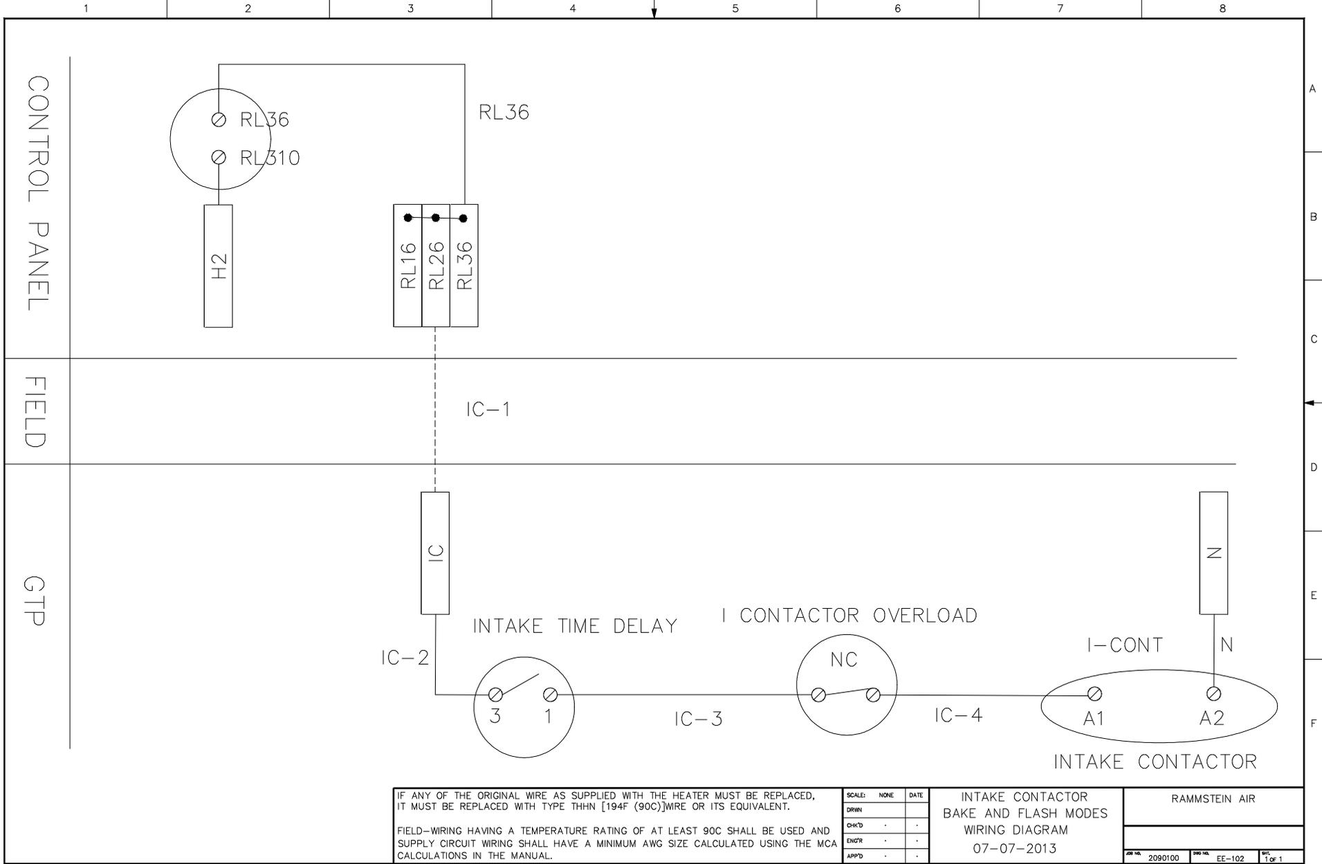
IF ANY OF THE ORIGINAL WIRE AS SUPPLIED WITH THE HEATER MUST BE REPLACED, IT MUST BE REPLACED WITH TYPE THHN [194F (90C)] WIRE OR ITS EQUIVALENT.
