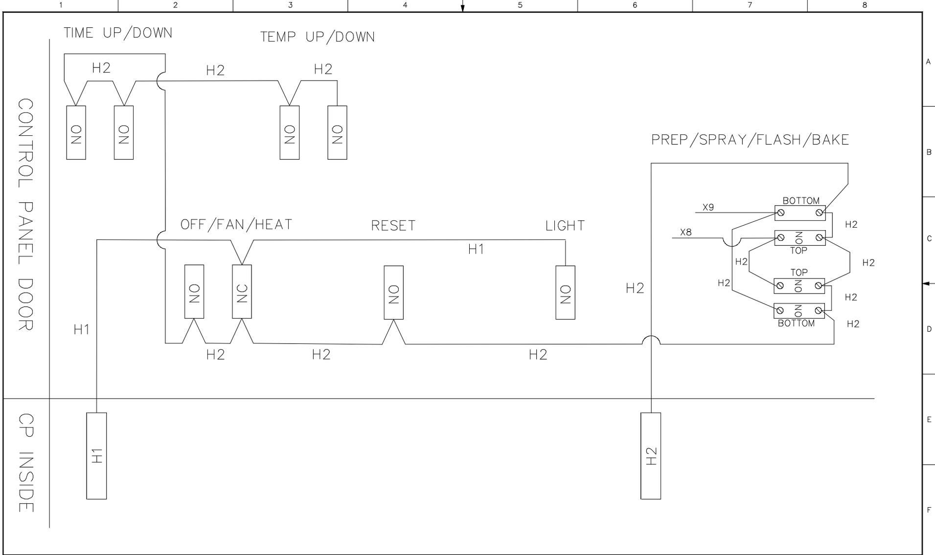
IF ANY OF THE ORIGINAL WIRE AS SUPPLIED WITH THE HEATER MUST BE REPLACED, IT MUST BE REPLACED WITH TYPE THHN [194F (90C)] WIRE OR ITS EQUIVALENT.
