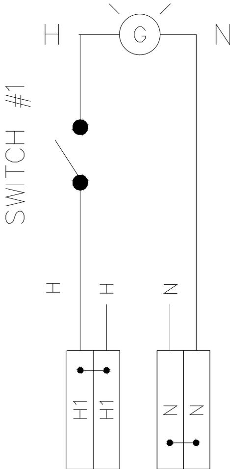
Now we can turn the light on and off when we want to. Let's say we only want the light on when the system ramped up to full air flow. This takes 5 seconds. We need a timer that delays the light coming on for 5 seconds. These timers are called on delay timers since they delay the activation of a device. There are also off delay times. As they name states these times delay the turning off or the deactivation of a device.
