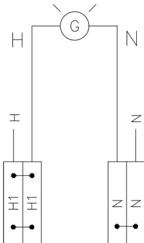
The above circuit is simply a circuit. It is probably the most basic form of a circuit. It is a circuit, but it is not a control circuit. We have no control over the light. If the power is on, the light will be on. To make it into a control circuit, let's wire in a switch.
