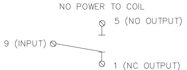
When the relay is turned on, the NC contact open and the NO set of contacts closes. If you have something connected to the NC contacts, it turns off. If you have something connected to the NO set of contacts, it will be turned on.
