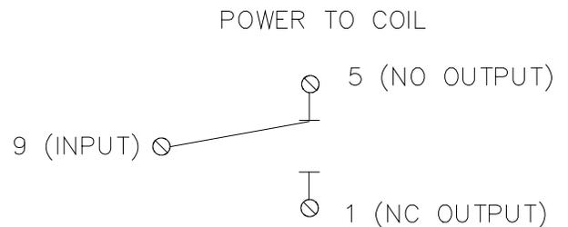
Take a look at the drawing. The signal goes in through 9. The signal can go to wither 1 or 5 depending on if the relay is energized or not. If the relay is not energized, 9 will be connected to 1 (NC terminal). If the relay is energized, 9 will switch to 5 (NO terminal). This means that when the relay is energized the signal will be present on the 5 terminal.
