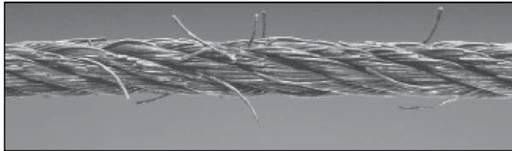
Cable with Corrosion
