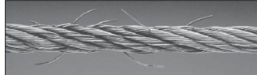
Cable with Broken Wires
