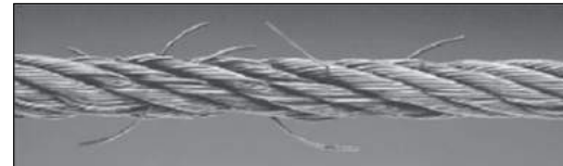
Cable with Broken Wires
