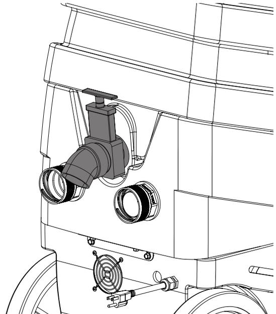
When the float shuts off vacuum, empty tank. Pull lever located at the back of the machine to release water.
