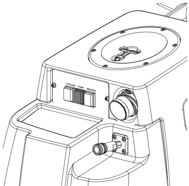
After the machine has been plugged into a 20 amp grounded outlet, turn on pump. Key tool until upholstery tool releases a steady flow.
