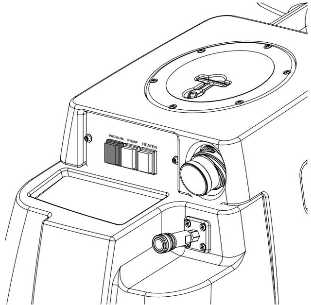
Turn on vacuum motor and begin cleaning. For best results make two dry passes to every wet pass.
