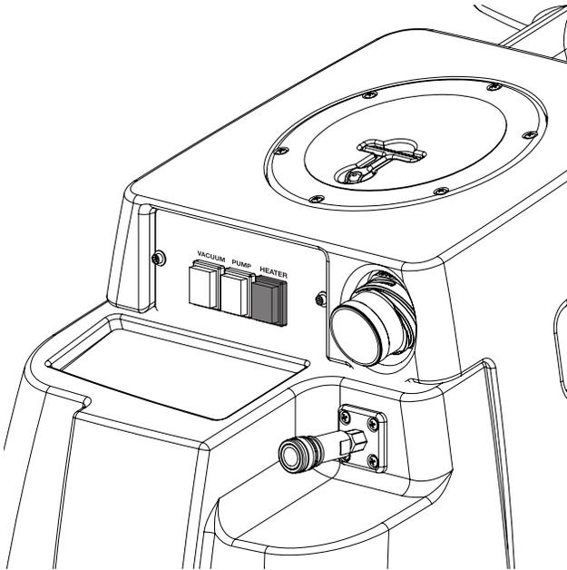
Release tool trigger. Turn on heater. Wait 8 – 10 minutes for unit to pre-heat. Once heated, re-key upholstery tool until hot water begins flowing. Once hot water is flowing, release trigger and pre-heat an additional 4 – 5 minutes.
