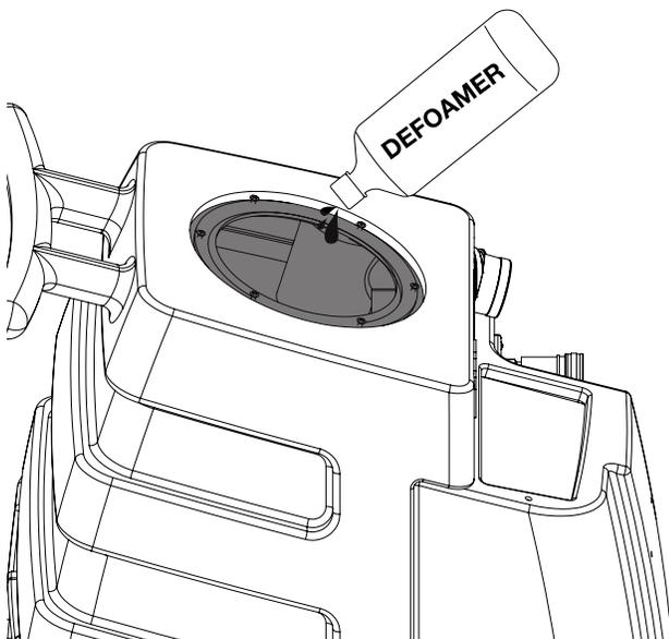
Add a defoamer in the recovery tank to reduce foam, prolonging the life of the Grand Prix™ vacuum motor.
