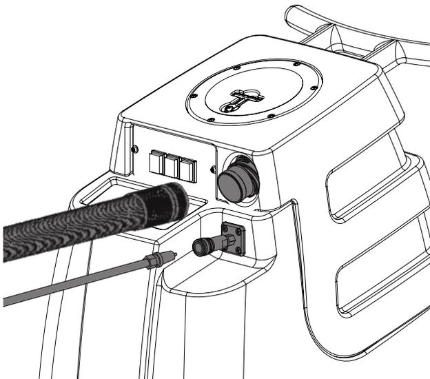
Attach one end of a solution hose to a wand or other tool, the other end to the Grand Prix™ front quick disconnect. Attach one end of a vacuum hose to the tool, the other end to the Grand Prix™ Cuff-Lynx™ vacuum hose port.
