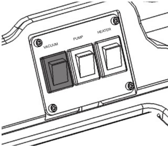
Turn on vacuum motor and begin cleaning. For best results make two dry passes to every wet pass.
