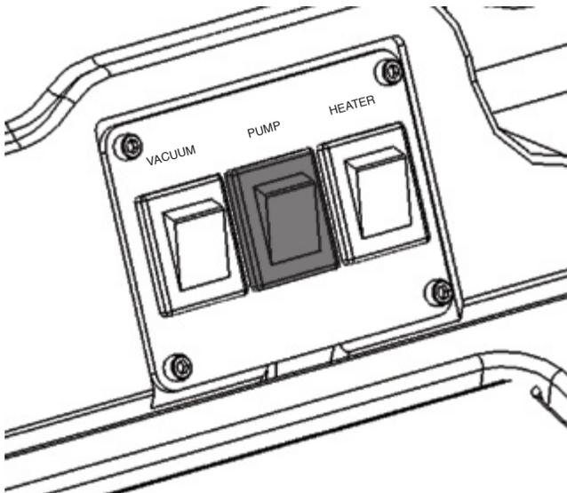
After the machine has been plugged into a 20 amp grounded outlet, turn on pump. Squeeze the trigger on the tool until it releases a steady flow.
