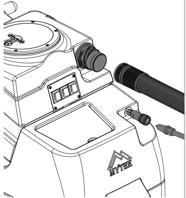
Attach one end of a solution hose to a wand or other tool, the other end to the Spyder's™ front quick disconnect. Attach one end of a vacuum hose to the tool, the other end to the Spyder's™ Cuff-Lynx™ vacuum hose port.
