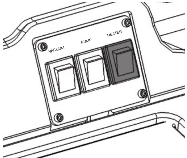
Release tool trigger. Turn on heater. Wait 8 – 10 minutes for unit to pre-heat. Once heated, re-key upholstery tool until hot water begins flowing. Once hot water is flowing, release trigger and pre-heat an additional 4 – 5 minutes.
