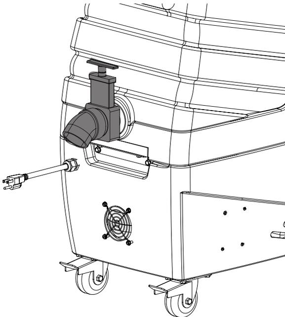
When the float shuts off vacuum, empty tank. Pull lever located at the back of the machine to release water.
