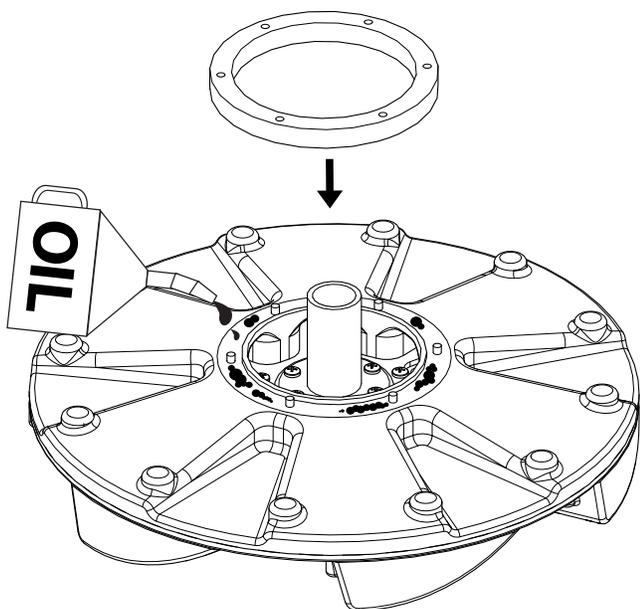
Make sure to keep your felt seal (Part # G014) lubricated. To do this, saturate the felt seal thoroughly with Mytee's lubricant (Part # PH648).
