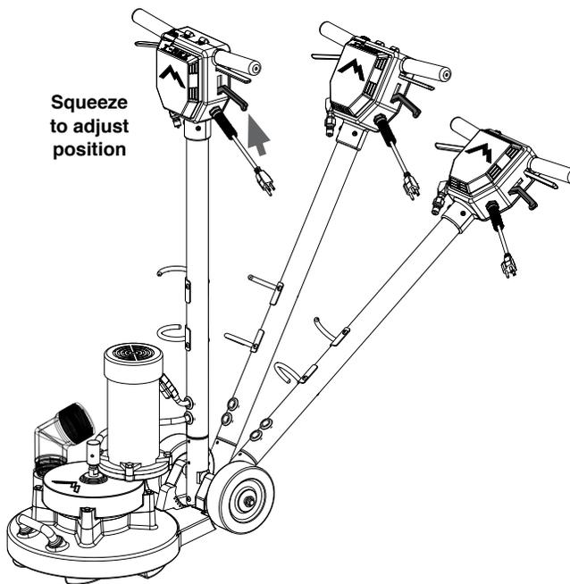
The handle can be adjusted to any desired working position by simply squeezing the adjustment lever. Move the handle to the desired position, then release adjustment lever locking handle in place.
