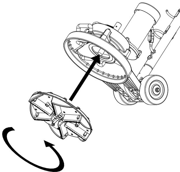
To attach the head, place the center piece of the head on the threaded piece located underneath, at the center of the T-REX™. Once on, twist counter-clockwise.
