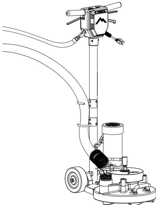
Connect solution hose from your extractor to swivel QD fitting on T-REX™ handle. Also, connect vacuum hose from extractor to Clear View Cuff-Lynx™ elbow or A105 lead hose.
