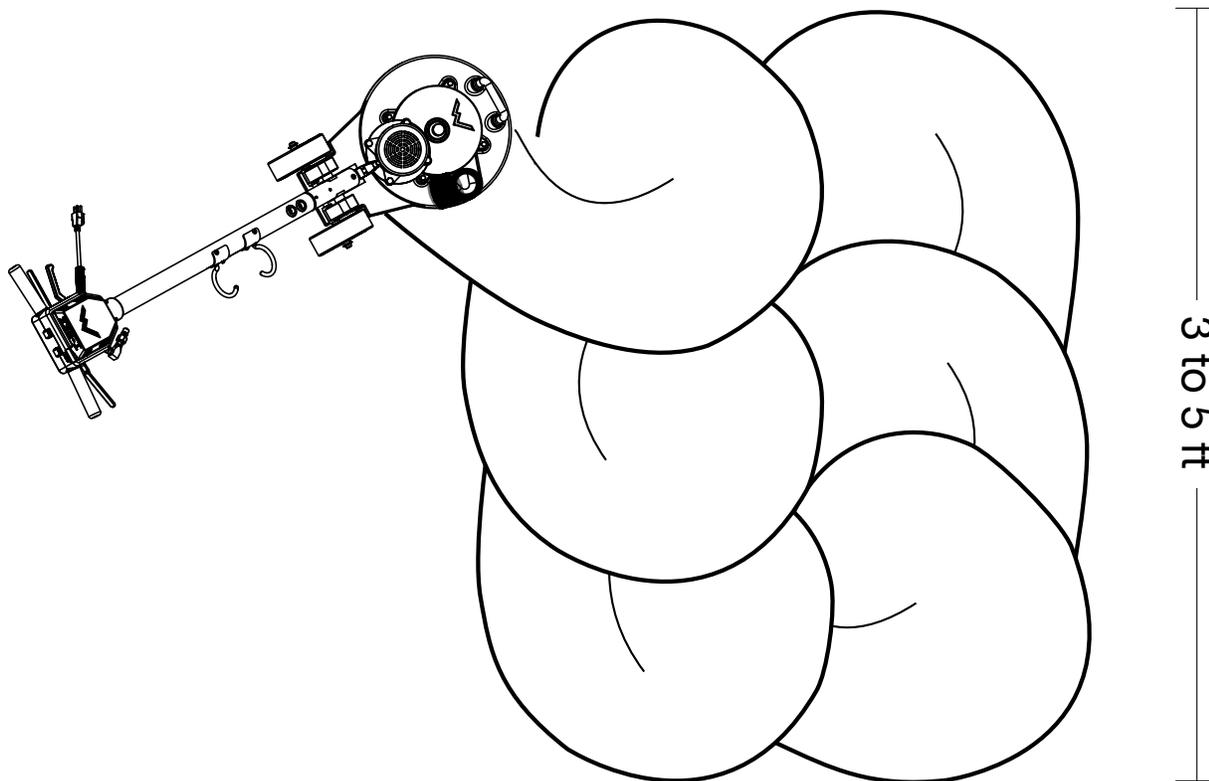
To get the best carpet cleaning results, move your T-REX™ in an arc pattern or circular motion. To remove stubborn stains, try hovering the T-REX™ over the stain.
