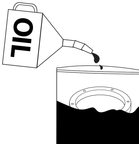
If you have run out of lubricant when it comes time to replace the felt seal, you may use a quality, 30 weight SAE motor oil in its place. Place the new felt seal in a bag along with some oil. Make sure that the entire felt seal is thoroughly lubricated.
