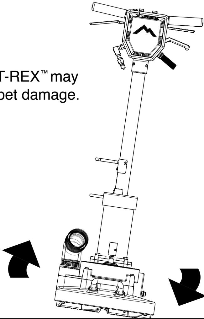
Your T-REX™ maneuvers much like a floor machine. Slightly lift handle to move to the right. Press the handle down slightly to move to the left. Tilting your T-REX™ may result in carpet damage. Remember to always keep T-REX™ evenly balanced on the surface.
