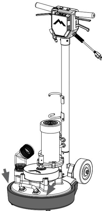
Head cover is protects the head from any type of damage. Simply press down on the head cover to remove. Apply cover when not in use.
