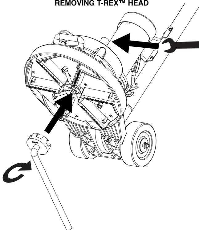
To remove, place wrench on rotary union and attach the head removal tool and twist clockwise.
