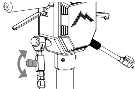
Turn the knob **counter-clockwise** for more flow to clean high-traffic areas. Turn **clockwise** for less flow to clean lower traffic areas.
