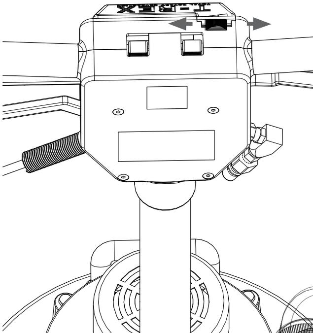
Located at the top of the unit is a speed adjuster. Unit adjusts from 80 - 160 RPM. Move to the left for a slower speed. Move to the right to speed up. Position to desired speed.
