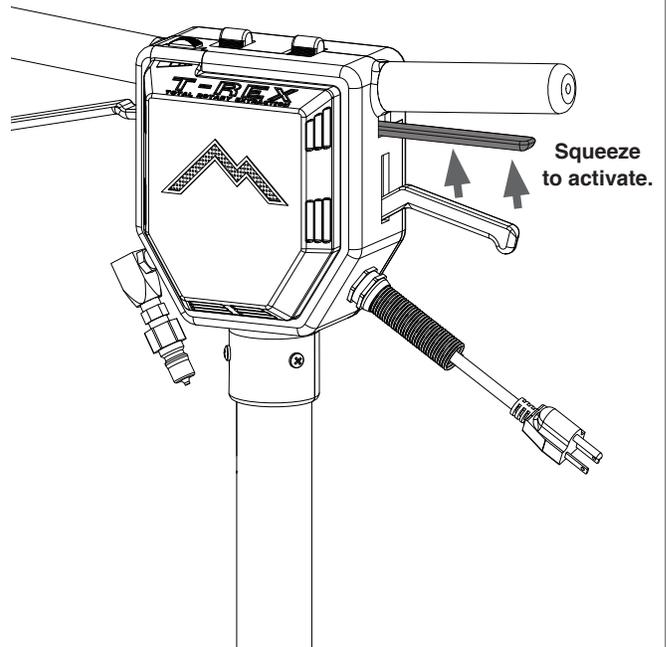
While holding the safety switch lock in disengaged position, squeeze the activation lever to operate machine. To stop the machine, simply release the lever.
