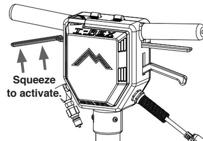
Squeeze lever for solution flow. PSI will be controlled by your extraction unit.
