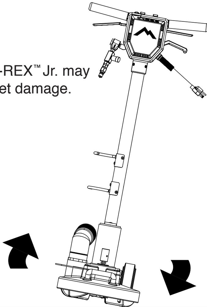
Your T-REX™ Jr. maneuvers much like a floor machine. Slightly lift handle to move to the right. Press the handle down slightly to move to the left. Tilting your T-REX™ Jr. may result in carpet damage. Remember to always keep T-REX™ Jr. evenly balanced on the surface.
