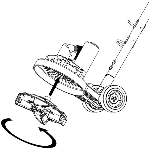
To attach the head, place the center piece of the head on the threaded piece located underneath, at the center of the T-REX™ Jr. Once on, twist counter-clockwise.
