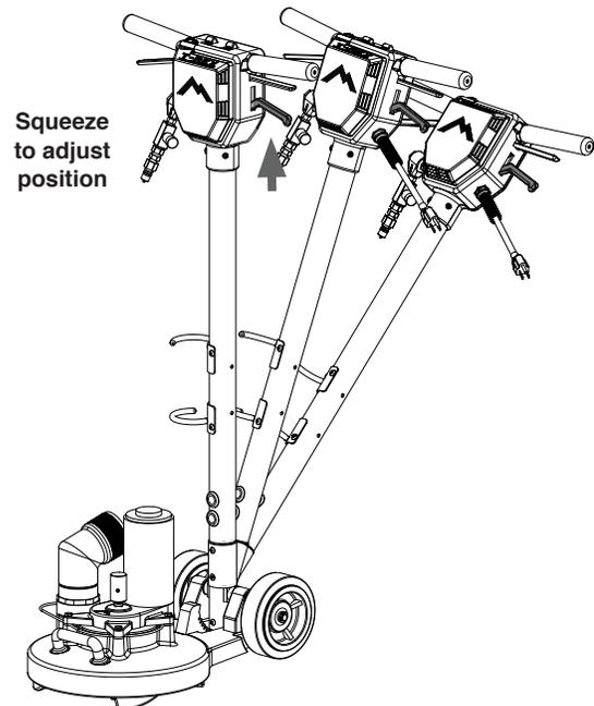
The handle can be adjusted to any desired working position by simply squeezing the adjustment lever. Move the handle to the desired position, then release adjustment lever locking handle in place.
