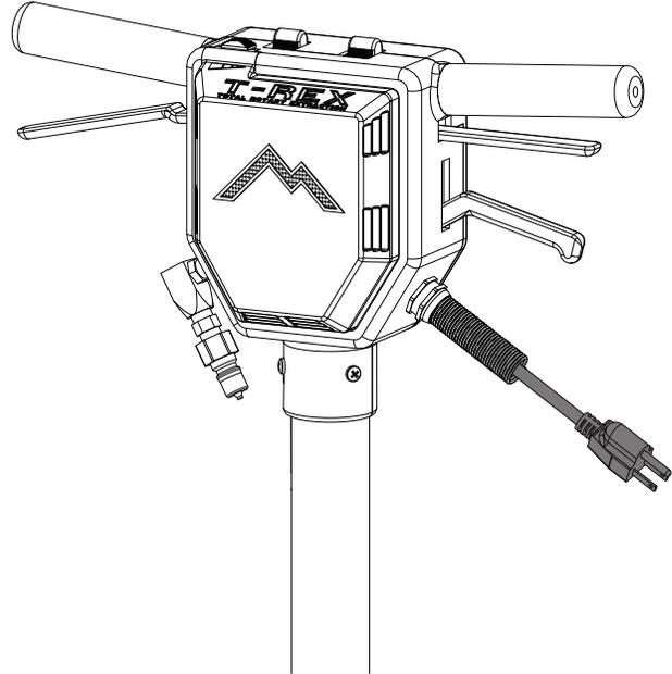
Connect pigtail plug to 25' power cord. Plug power cord into a grounded wall outlet.
