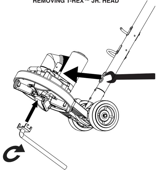
To remove, place wrench on rotary union and attach the head removal tool and twist clockwise.
