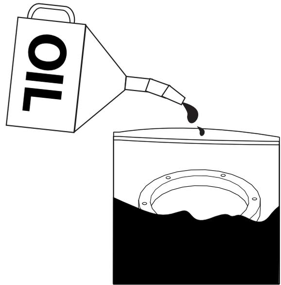
If you have run out of lubricant when it comes time to replace the felt seal, you may use a quality, 30 weight SAE motor oil in its place. Place the new felt seal in a bag along with some oil. Make sure that the entire felt seal is thoroughly lubricated.
