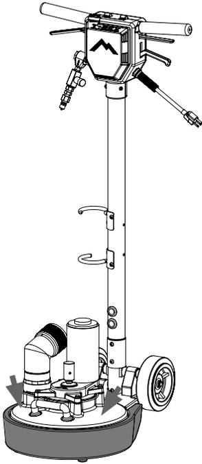
The head cover protects the head from any type of damage. Simply press down on the head cover to remove. Apply cover when not in use.
