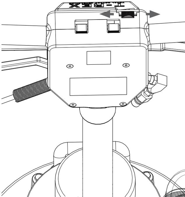
Located at the top of the unit is a speed adjuster. Unit adjusts from 80 - 180 RPM. Move to the left for a slower speed. Move to the right to speed up.
