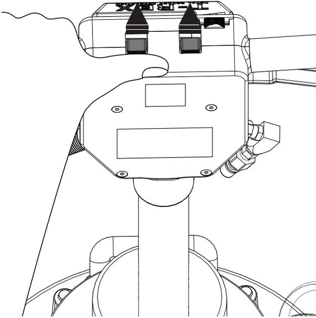
The handle must be lowered to the operating position before switching the machine ON. Disengage the safety switch lock by pushing it forward with either thumb.
